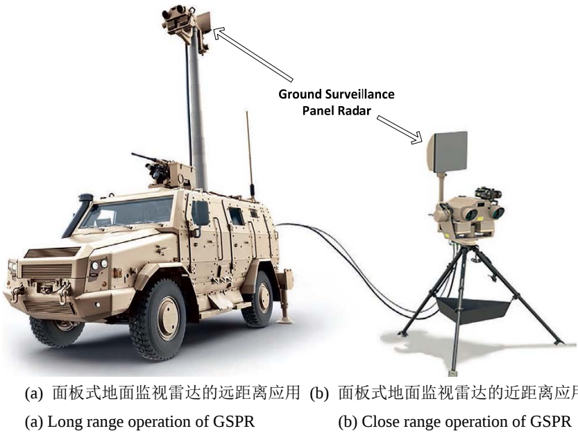
图 9 面板式地面监视雷达安装在车载光电桅杆上和车辆附近的三脚架上 Fig.9 Ground Surveillance Panel Radar (GSPR) mounted on vehicle electro-optic mast and tripod away from vehicle
