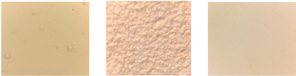
(a) A 腐蚀液 (a) A corrosion solution (b) B 腐蚀液 (b) B corrosion solution (c) AB 腐蚀液 (c) AB corrosion solution
