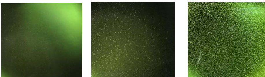
(a) 4.5 N 时芯片表面 (b) 9 N 时芯片表面 (c) 13.5 N 时芯片表面 (a) Chip surface when the pressure is 4.5 N (b) Chip surface when the pressure is 9 N (c) Chip surface when the pressure is 13.5 N
