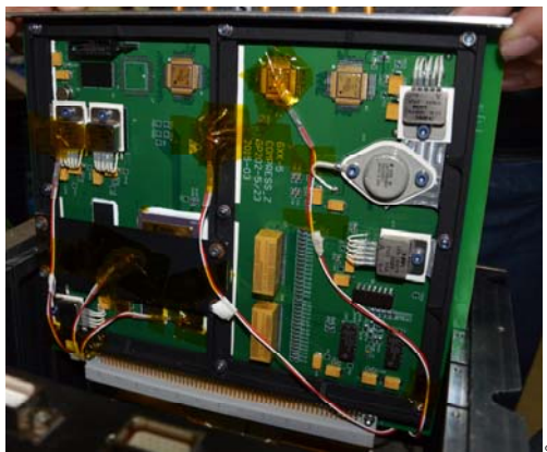
图 6 电控箱放置测温电阻 Fig.6 Temperature resistances in electric cabinet
