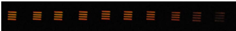
图 10 AOTF 频率固定, 靶标图像随调制幅度增大的变化 Fig.10 The change of the target image, when the AOTF frequency is fixed
