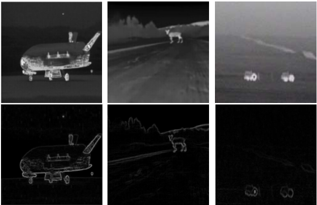
图 8 本文改进边缘提取算法在红外目标探测领域的应用 Fig.8 The application of the improve algorithm in the infrared target detection
