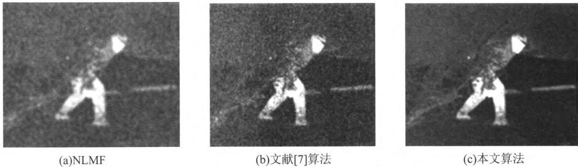
图 4 添加方差为 15 的高斯噪声图像滤波结果对比 Fig.4 Comparison of the filtering results of the Gaussian noise image with the variance of 15
