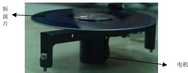
图1 斩波器外形图 Fig.1 Outside view of chopper
