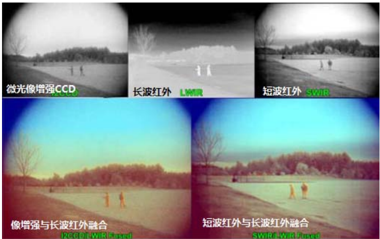
图10 采用I 2 CCD作为VNIR通道的VNIR/LWIR的双探测器的图像融合,和采用InGaAs FPA作为SWIR通道的SWIR/LWIR双探测器的图像融合,均采用非制冷微测辐射热计作为LWIR通道 Fig.10 Dual-sensor fusion of VNIR/LWIR using an I 2 CCD for the VNIR channel, and SWIR/LWIR using an InGaAs FPA for the SWIR channel, both using an uncooled microbolometer for the LWIR channel
