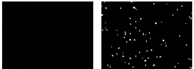
图 4 死像元分布图像 图 5 阈值检测结果 Fig.4 The distributing image of the blind pixels Fig.5 The result of threshold detection
