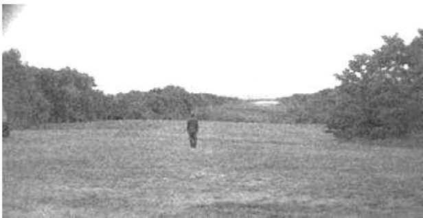
图 9 采用 InGaAs 相机在无月亮条件下对人的成像效果 Fig. 9 Image capture on a dark, moonless night using the MANTIS digital camera operating at a 30 Hz frame rate with a f/1.4 lens
