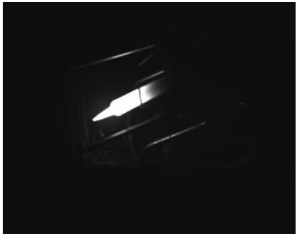
图7 采用320×256 InGaAs像机测试得到的电烙铁加热过程的热辐射成像 Fig.7 Hot radiation image of hot iron during warming process taken by 320×256 InGaAs camera
