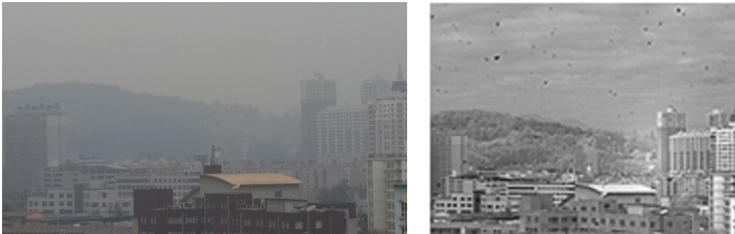
图 8 采用可见光相机(左)和 320×256 InGaAs 相机(右)在有雾条件下的成像效果 Fig.8 Pictures of the same scene taken with a visible camera (left) and 320×256 InGaAs camera (right)
