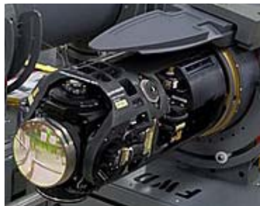
图4 狙击手增程型瞄准吊舱三光共孔径前视红外传感器 Fig.4 Sniper XR (Extended Range) targeting pod three optical common aperture FLIR sensor
