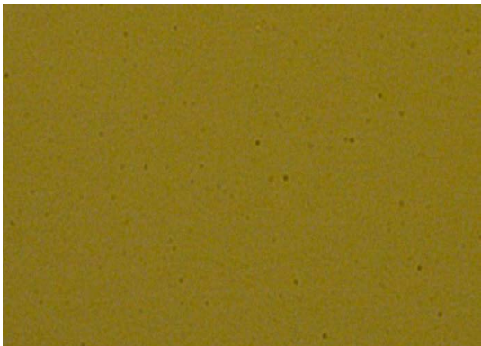
图 6 粘接胶固化后无气泡的粘接界面显微照片 Fig.6 The microscope photo of bonding interface without bubbles after adhesive glue curing
