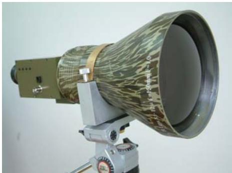
图 12 一种光学镜头焦距为 150 mm 的非制冷热成像仪 Fig.12 An uncooled thermal imager with 150 mm lens focal length
