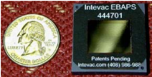
图 17 Intevac 研发的 EBAPS Fig.17 EBAPS developed by Intevac
