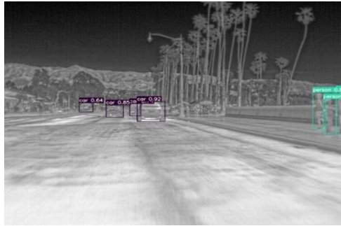
(c) YOLOv7s 在复杂背景下的检测效果 (c) YOLOv7s detection effect in complex backgrounds
