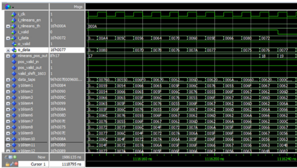
图5 红外图像算法处理仿真波形数据 Fig.5 Infrared image algorithm processing simulation waveform data
