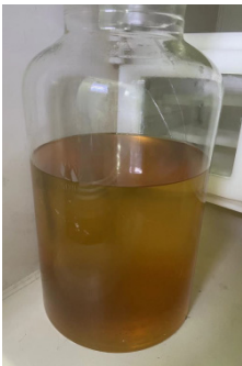
(a)硝棉溶于乙酸丁酯第 1 天 (b) 硝棉溶于乙酸丁酯第 7 天 (a) Diagram of Nitrocellulose dissolved in Butyl Acetate on the first day (b) Diagram of Nitrocellulose dissolved in Butyl Acetate on the seventh day
