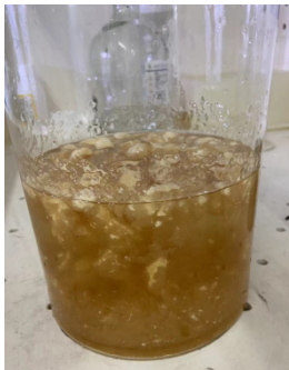
(a)硝棉溶于乙酸丁酯第 1 天 (b) 硝棉溶于乙酸丁酯第 7 天 (a) Diagram of Nitrocellulose dissolved in Butyl Acetate on the first day (b) Diagram of Nitrocellulose dissolved in Butyl Acetate on the seventh day
