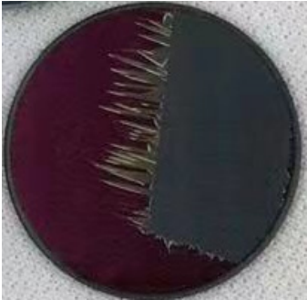
图3 附着力测试结果 Fig.3 The results of adhesion test
