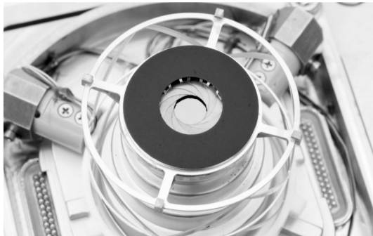
图 10 雷神公司可变冷光阑杜瓦俯视图 [16] Fig.10 View of top of variable aperture cold shield installed in sealed tactical dewar from Raytheon [16]
