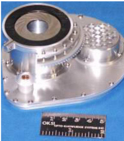
图 7 外置可变光阑与滤光片转盘的集成结构 [11] Fig.7 The integrated structure of variable-aperture mechanism (VAM) and cold filter wheel [11]
